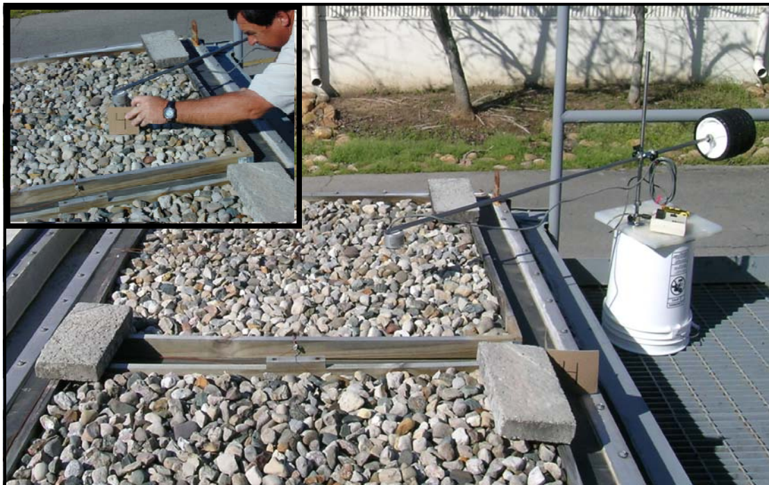
Figure 5. Use of a custom-made albedometer to measure the solar reflectance of the 4 ft square stone-ballasted test sections. Inset shows adjustment of the height of the albedometer to 4 in. above the stone surface.
