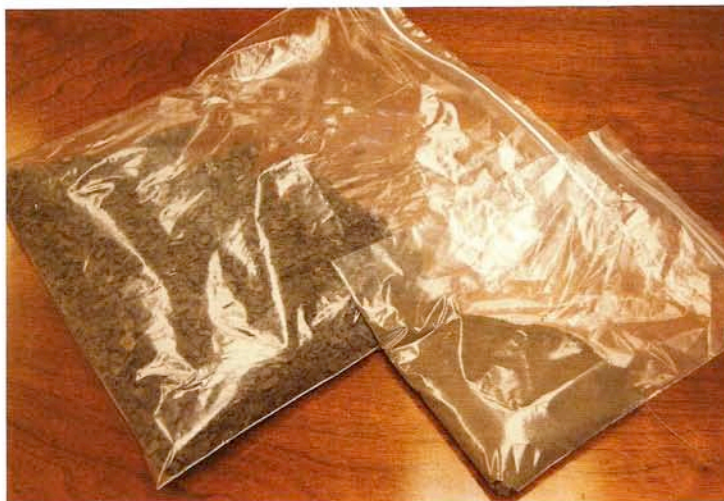
An EPDM membrane following the grinding process
