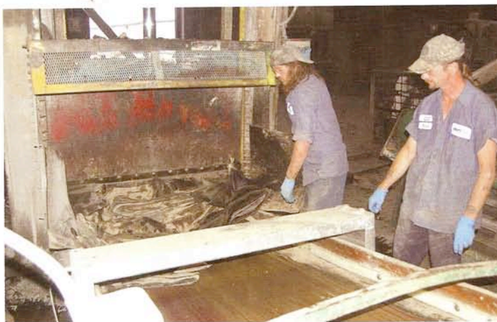
An EPDM membrane is ground at Midwest Elastomers Inc.'s grinding facility in Wapakoneta, Ohio.
