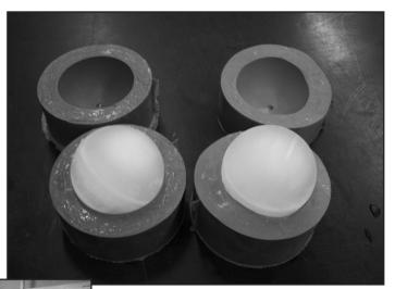
lets (ice spheres) require precise fabrication in order to achieve reproducible impact energies.
