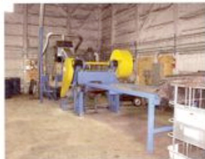
■ At WDG's facility in LaGrange, Ohio, 5-foot by 5-foot sheets of EPDM are sheared and ground into crumb rubber.
